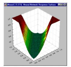
The figure above shows the plateau response surface developed by an MLP to solve the XOR problem: as can be seen, this neatly sections the space along a diagonal.
