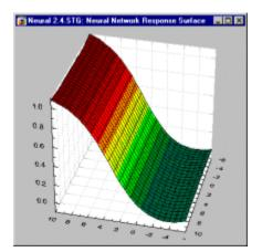
A multi-layered network combines a number of these response surfaces together, through repeated linear combination and non-linear activation functions. The next figure illustrates a typical response surface for a network with only one hidden layer, of two units, and a single output unit, on the classic XOR problem. Two separate sigmoid surfaces have been combined into a single U-shaped surface.
