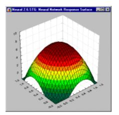
MLP units are defined by their weights and threshold, which together give the equation of the defining line, and the rate of fall-off of the function from that line. Before application of the sigmoid activation function, the activation level of the unit is determined using a weighted sum,
