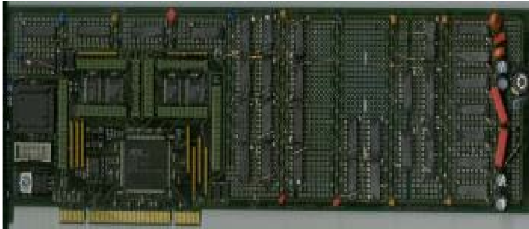
Figure 1.3: A PCI version generating true random numbers at 160 MByte/s [19]
